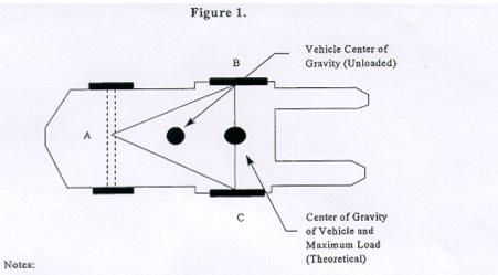
When the vehicle is loaded, the combined center of gravity (CG) shifts toward line B-C. Theoretically
